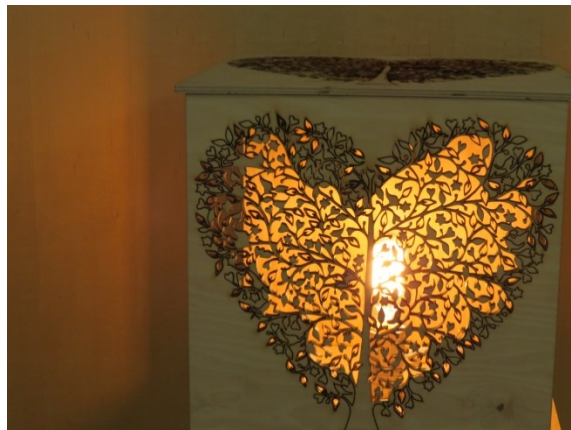
Laser-engraved heart on the front panel of a light box
